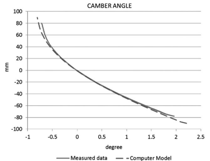
**Figure 9.** Camber - computer model validation.
