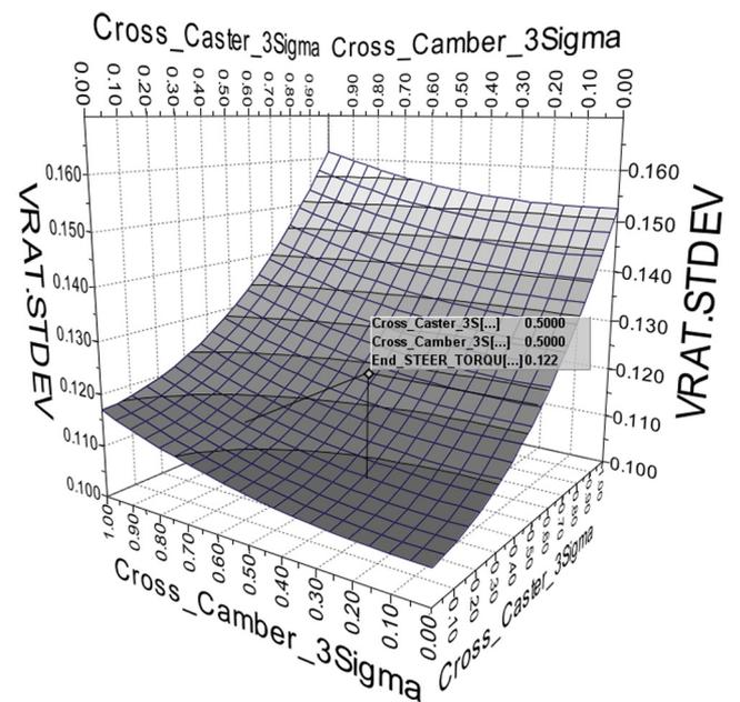
Figure 14. Cross camber and cross caster standard variation effects on VRAT standard variation.
