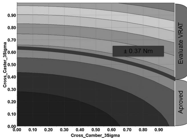
Figure 16. Example of final line checking graph for VRAT.
