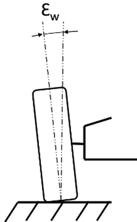
Figure 2. SAE Standard for positive camber angle.
