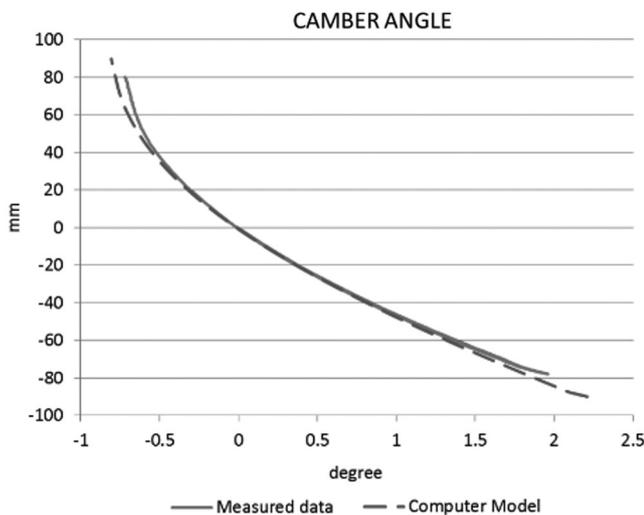
Figure 11. Suspension rate - computer model validation.
