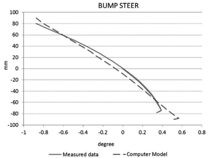
**Figure 8.** Bumper Steer - computer model validation.
