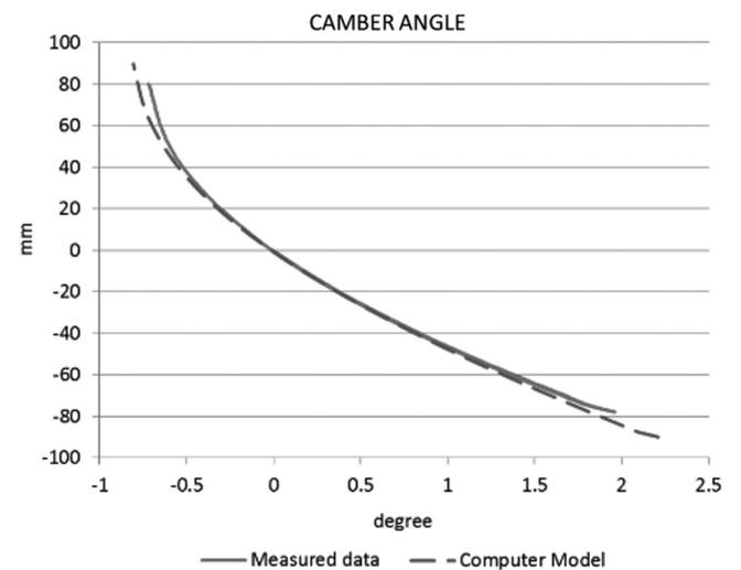
**Figure 9.** Camber - computer model validation.
