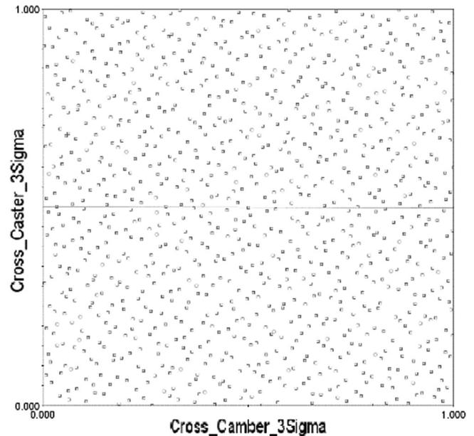
Figure 13. Sobol algorithm applied on cross camber and cross caster standard deviation.
