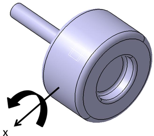
Figure 7. Tire conicity effects on momentum.
