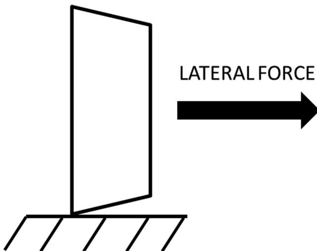
Figure 6. Tire conicity representation.
