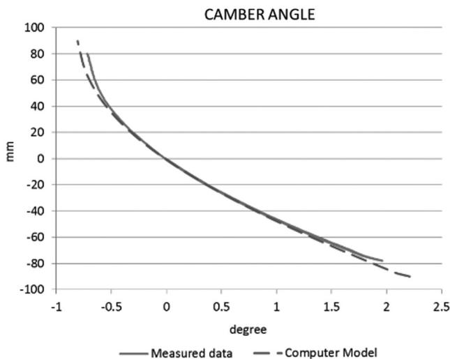
Figure 11. Suspension rate - computer model validation.
