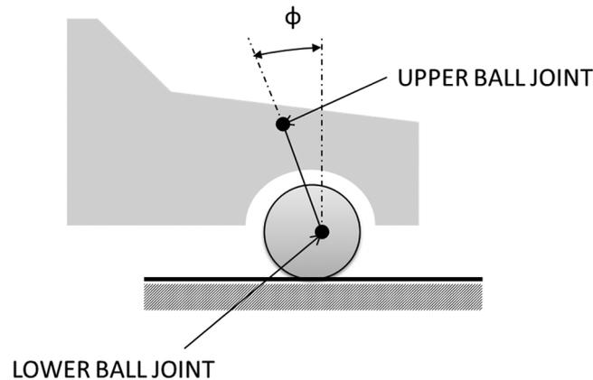
Figure 4. SAE Standard for positive caster angle.
