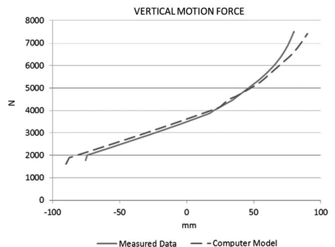
**Figure 10.** Vertical motion force - computer model validation.
