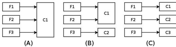
**Figure 1.** Totally integral (A), modular focus (B) and totally modular (C) product architectures.
