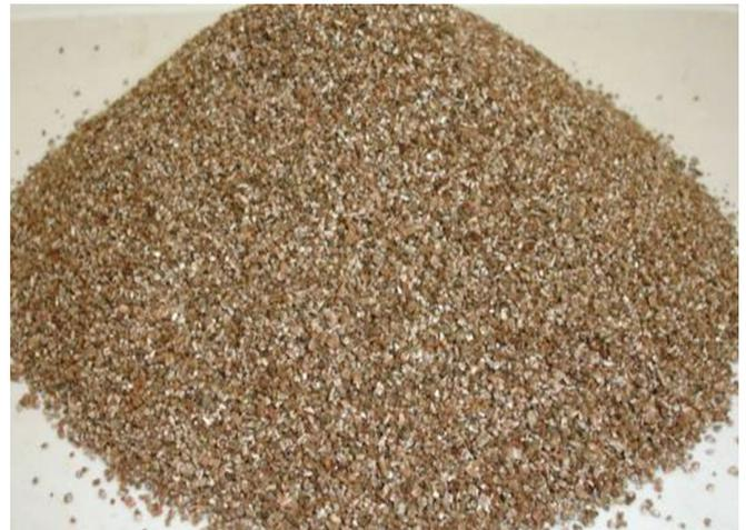
**Figure 1.** Expanded Vermiculite. Source: Melo et al. (2012).
