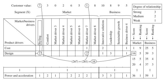
**Figure 18.** Illustration of the analysis and prioritization of the product requirements in the House of Quality method for the development of a passenger car (adapted from PHAAL et al., 2003a).
